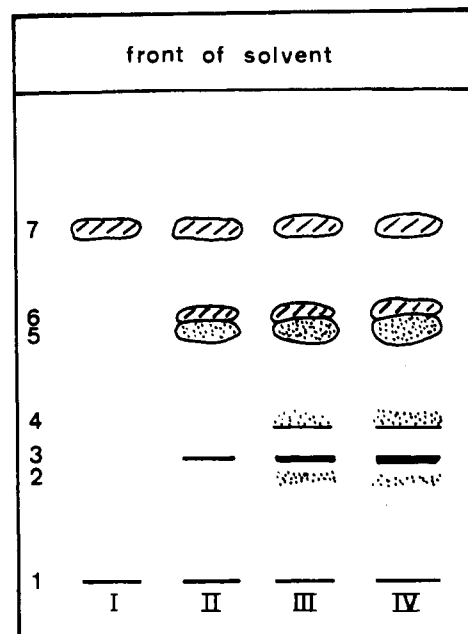
Figure 8. Nonvolatile compounds produced after heat treatment of \beta -carotene at 97 °C for different times [I, 0 h; II, 1 h; III, 2 h; IV, 3 h] and separated by TLC on aluminum oxide F 254 type T: 1, starting; 2, aurochrome; 3, mutatochrome; 4, nonidentified; 5, neo-T-5,6,5',6'-diepoxy- \beta -carotene; 6, 5,6-epoxy- \beta -carotene; 7, \beta -carotene.
